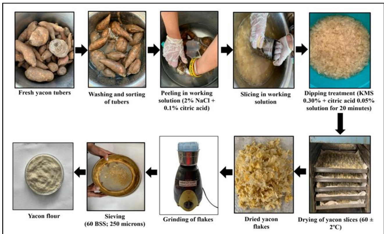
Figure 1: Unit operations for the preparation of flour from Yacon tubers.
