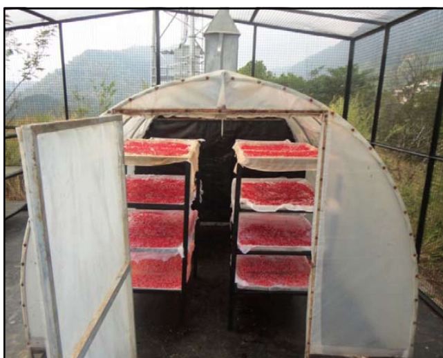
Figure 1: Drying of wild pomegranate arils for anardana preparation under solar tunnel drier.
