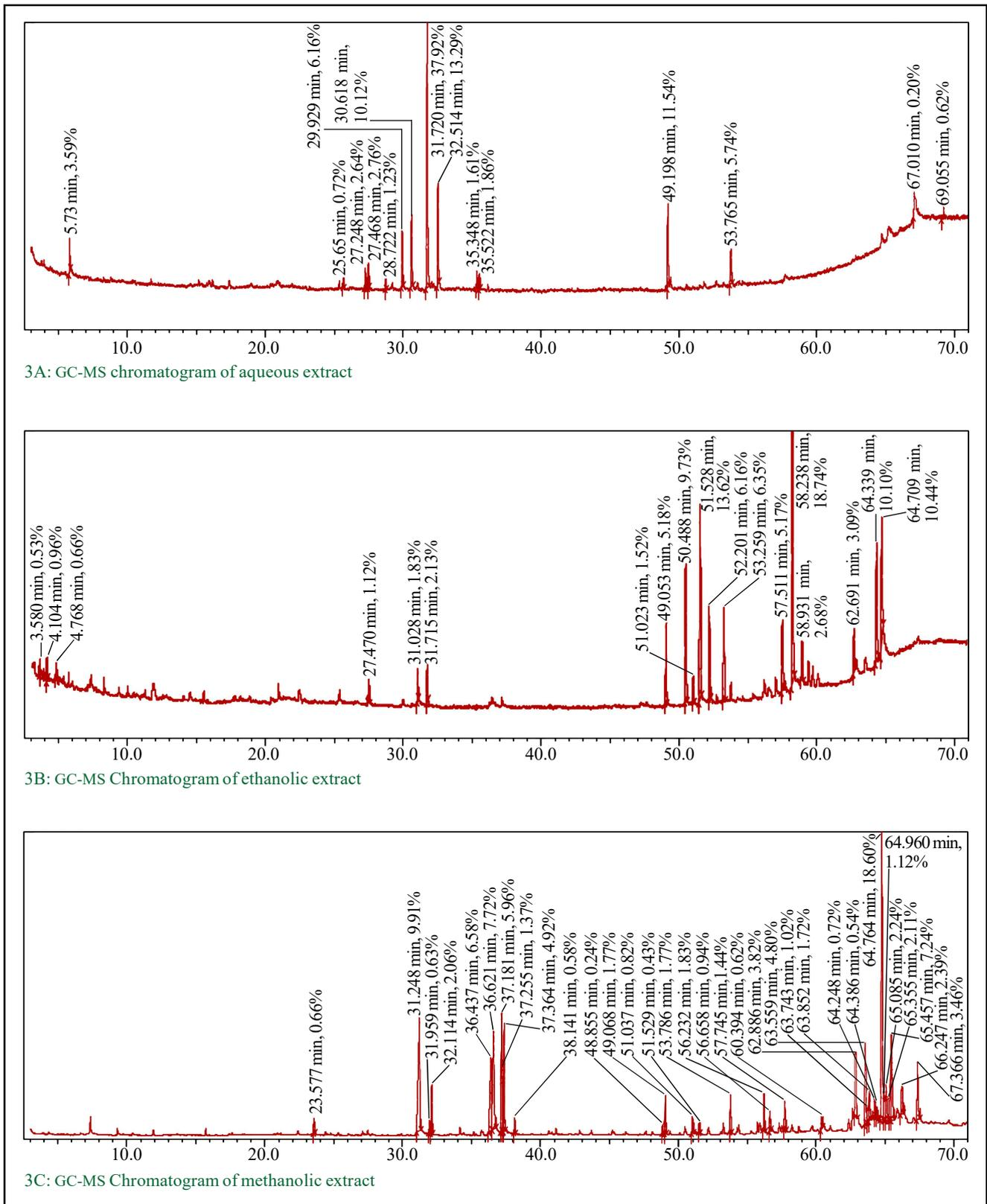
Figure 3: GC-MS Chromatogram of aqueous, ethanolic and methanolic extracts of *T. codifolia*.
