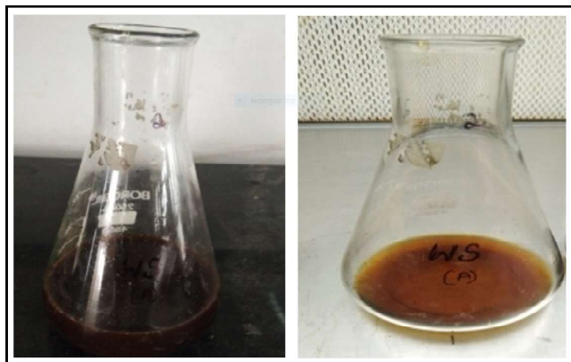
Figure 1: Synthesis of silver Nanoparticles: Visual observation of the change in the reaction mixture from greenish to brown colour upon addition of silver nitrate solution.
