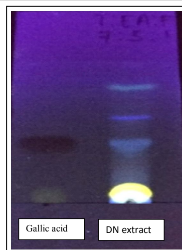
Figure 4(b): TLC of Gallic acid, present in DN leaf extract.
