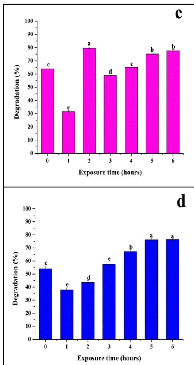
**Figure 4:** Degradation efficiency of TiO<sub>2</sub> NPs synthesized using *A. altissima* leaf extract on photocatalytic activity against: (a) methylene blue, (b) methyl orange, (c) crystal violet, and (d) alizarin red dyes. Different letters on each error bar are statistically significant at  $p \geq 0.05$  level.
