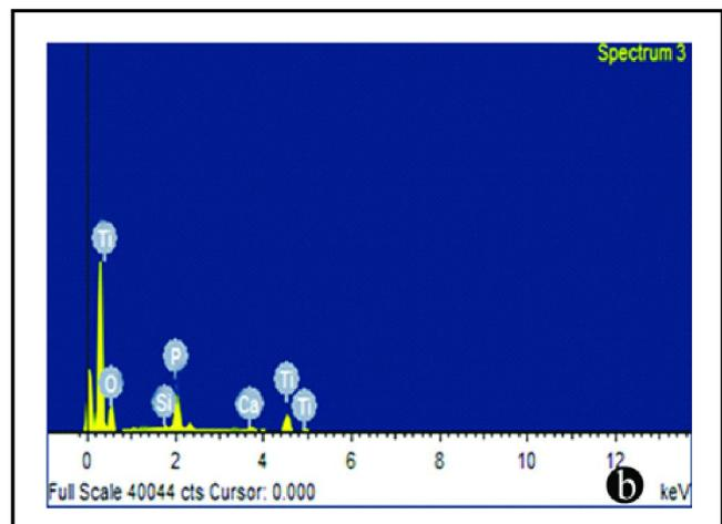
**Figure 3:** a) Field emission scanning electron microscopy (FESEM) image of spherical shape  $\text{TiO}_2$  nanoparticles and b) Energy dispersive X-ray (EDX) analysis showing strong  $\text{TiO}_2$  peaks.
