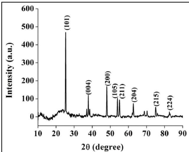
**Figure 2:** XRD pattern indicates the polycrystalline form of  $\text{TiO}_2$  NP.
