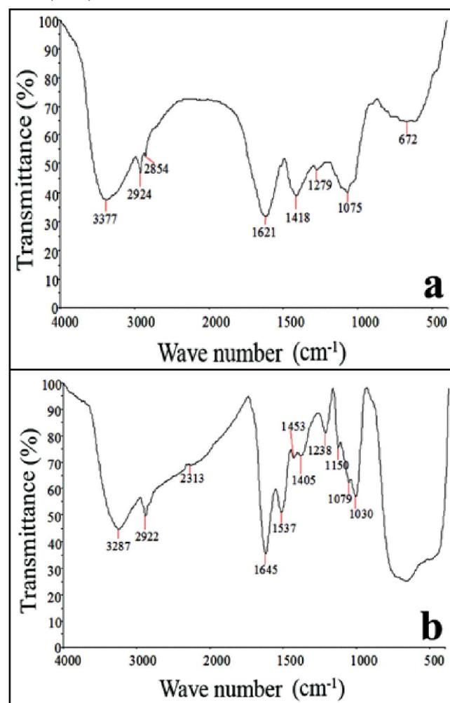
**Figure 1:** Fourier transform infrared spectroscopy analysis (FTIR) showing peaks for: a) aqueous leaf extract and b) biosynthesized  $\text{TiO}_2$  nanoparticles.
