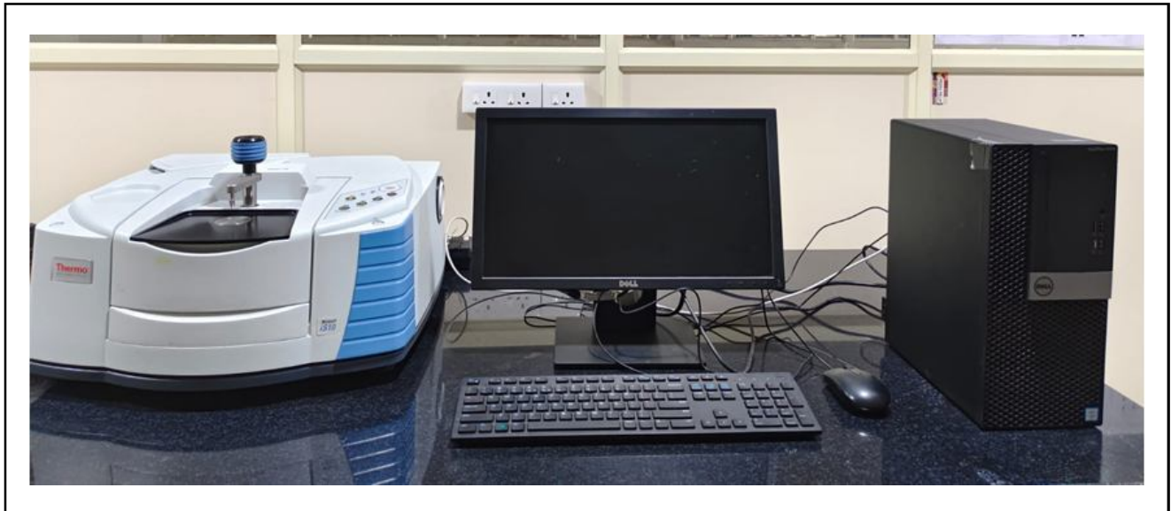
Figure 1: Image of the fourier transform infrared spectroscopy (Nicolet iS10 spectrometer) used for analysis.
