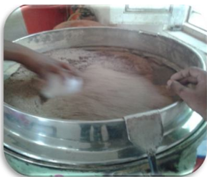
Figure 3: Pulverizing the coarse powder in a pulverizer and sieving the powder.
