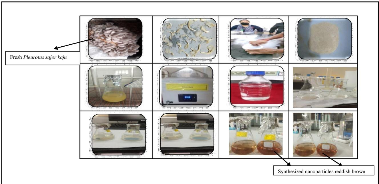
**Figure 1: Synthesis of silver nanoparticles: Visual observation of the change in the reaction mixture from yellowish to reddish brown colour upon addition of silver nitrate solution.**
