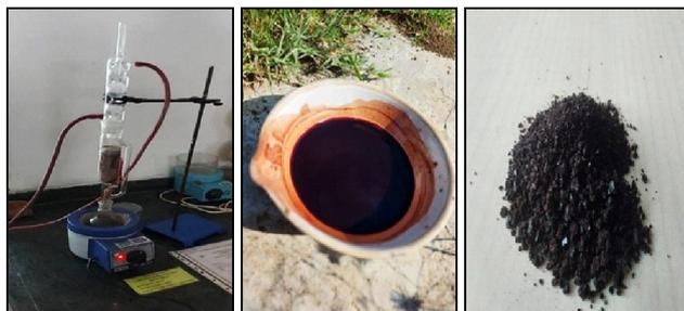
Figure 2: Synthesis of zinc oxide nanoparticle.
