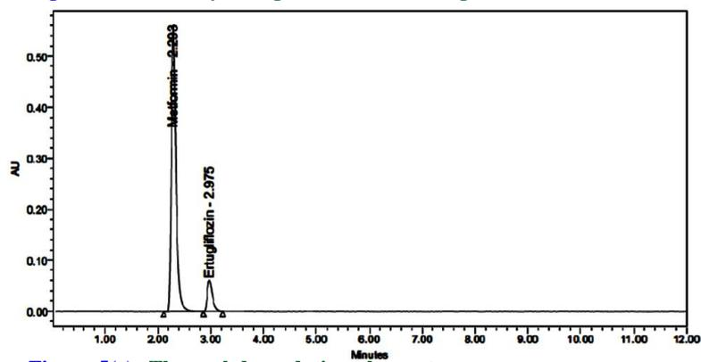
Figure 5(e): Thermal degradation chromatogram.
