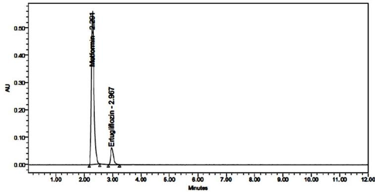
Figure 5(d): Photolytic degradation chromatogram.
