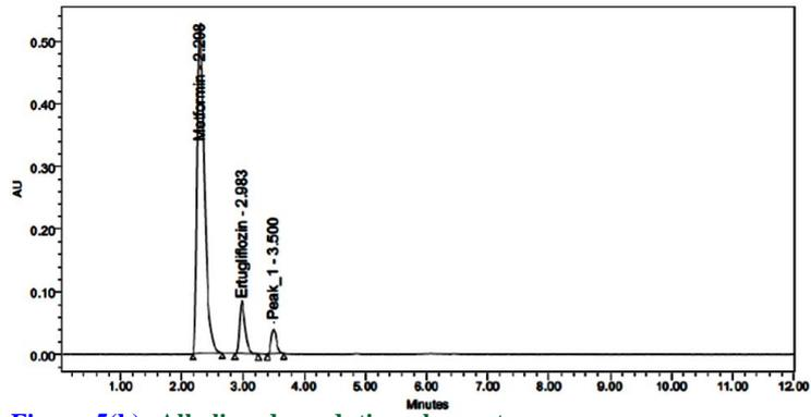
Figure 5(b): Alkaline degradation chromatogram.
