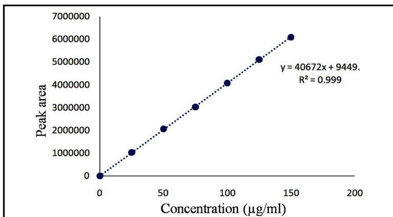
**Figure 4 (a): Linearity plot of metformin hydrochloride.**
