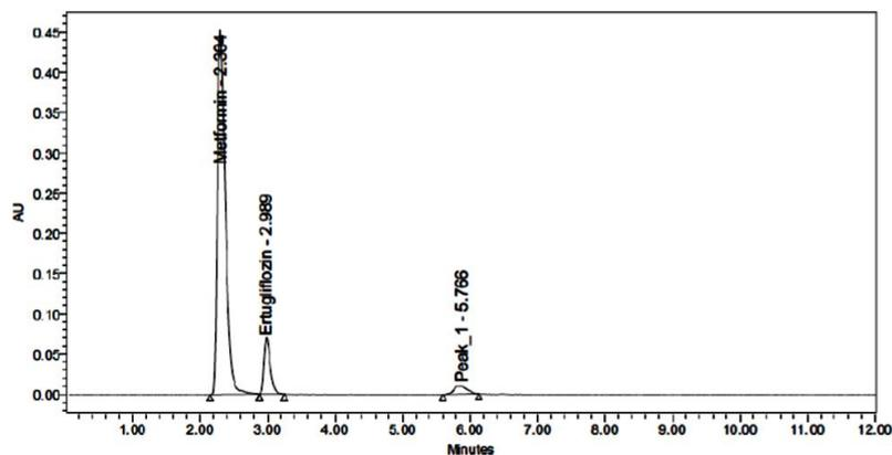
Figure 5(a): Acid degradation chromatogram.
