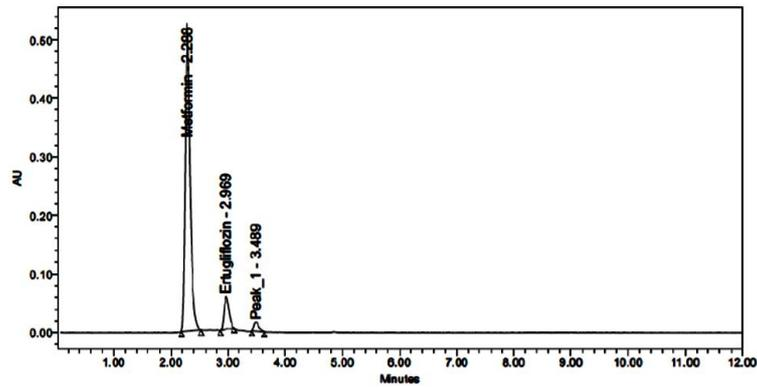
Figure 5(c): Oxidative degradation chromatogram.
