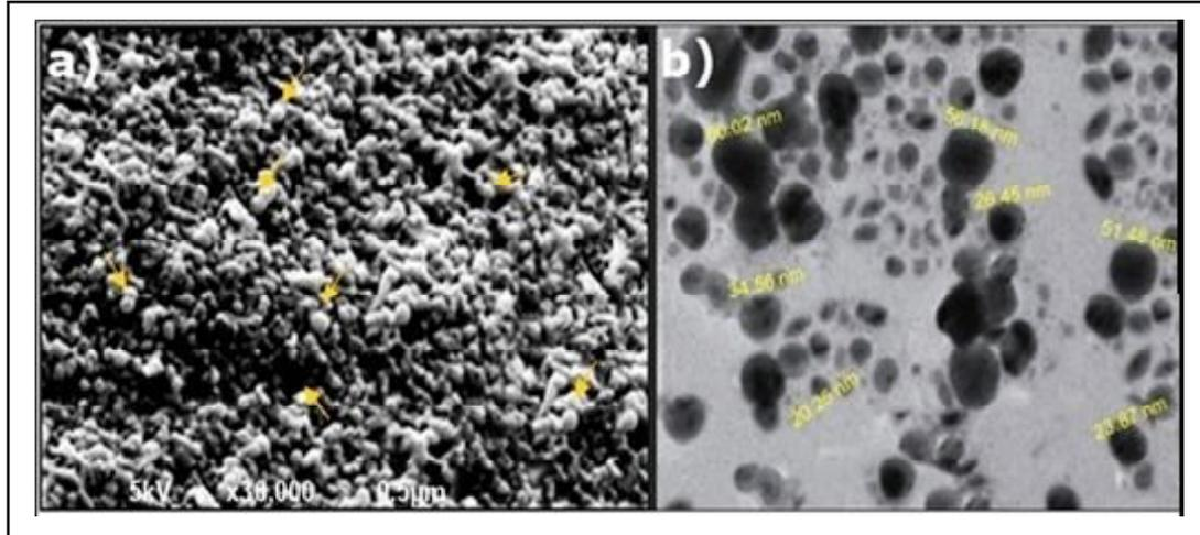
**Figure 5: (a) SEM image and (b) TEM image of AgNPs synthesized using seed extract of *N. sativa*.**
