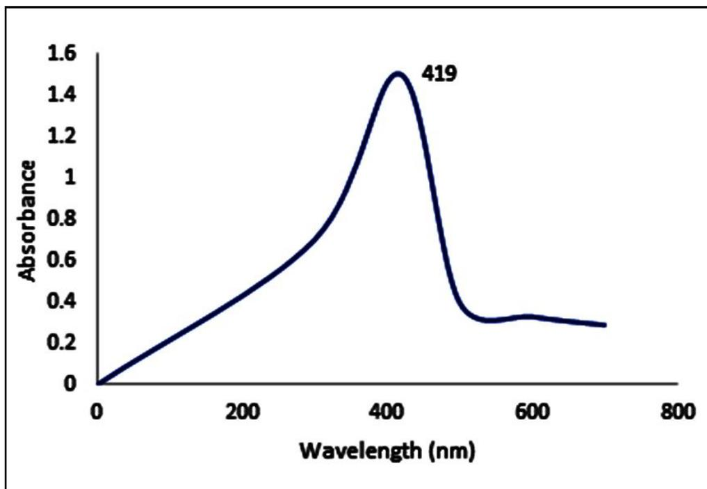
Figure 1: UV-Vis spectrophotometry of silver nanoparticles synthesized using *N. sativa*.
