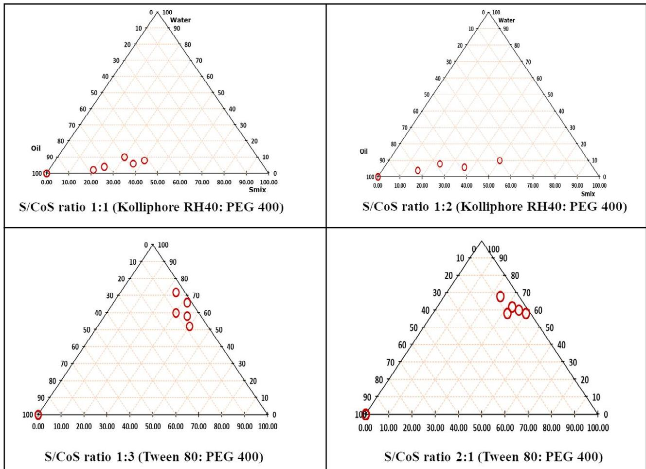
**Figure 1:** Pseudoternary phase diagrams system containing the following components: Sefsol 218 as oil, Kolliphor RH40 as a surfactant, PEG 400 as co-surfactant. The dotted area shows the nanoemulsion region in different ratios of surfactant to cosurfactant in 1:1, 1:2, 1:3, and 2:1.
