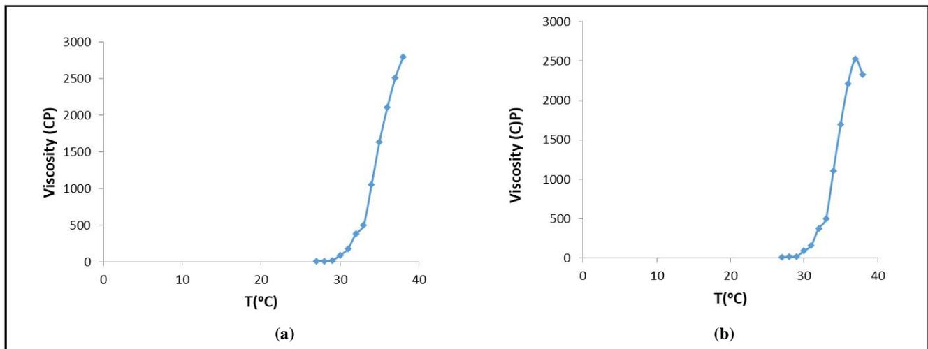
**Figure 2: Rheological flow curves of optimized *in situ* gel formulations (a) ISG16 and (b) ISG 17 at different temperatures.**
