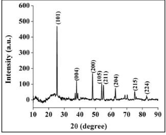
Figure 2: XRD pattern indicates the polycrystalline form of TiO, NP.
