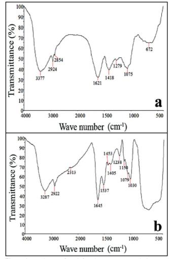
Figure 1: Fourier transform infrared spectroscopy analysis (FTIR) showing peaks for: a) aqueous leaf extract and b) biosynthesized TiO, nanoparticles.
