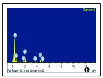
**Figure 3:** a) Field emission scanning electron microscopy (FESEM) image of spherical shape TiO<sub>2</sub> nanoparticles and b) Energy dispersive X-ray (EDX) analysis showing strong TiO<sub>2</sub> peaks.
